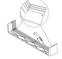
On a protected surface, carefully score down both corners to the desired cutoff point and snap to remove the excess.
