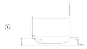
Measure the distance from the floor to the base of the lower door panel. Refer to the table below for the recommended cut location.
