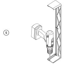
Punch or drill out the two mounting holes with a 5mm drill bit on each side of the toe kick as shown.
