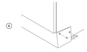
Secure toe kick to the Dishdrawer using the supplied pins.
