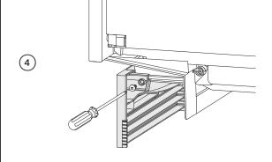
Slide toe kick onto the mounting rails and secure
