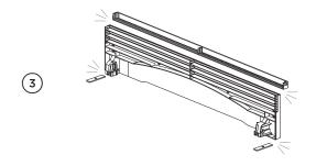
Snap excess + smooth edges. Snap both end tabs.
