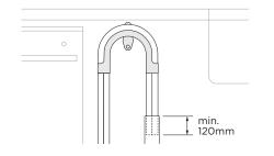
Pull both hoses through the support guide and rest in standpipe.
