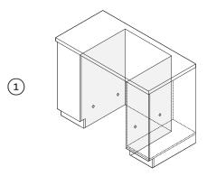
If securing via the drawer removal method, ensure the marked locations provide adequate support.
