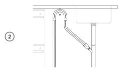
Pull both hoses through the drain hose support before threading the wire clips on to the hoses and fitting to the supplied hose joiner. Secure using the wire clips.
