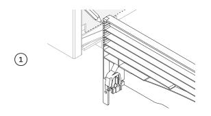
Measure toe kick height. Where the toe kick meets the bottom of the tub is the recommended cut-off point.
