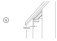
Align the supplied moisture protection tape to the cabinetry as illustrated
